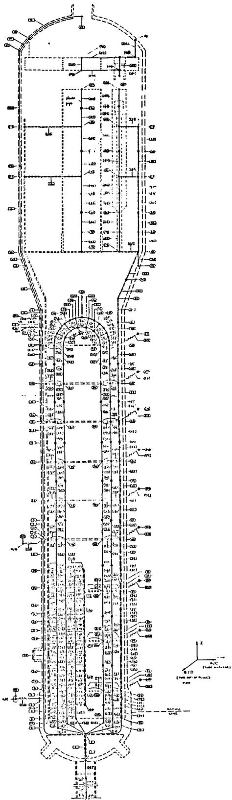
Figure 3b: Mathematical model of steam generator and its internals.
