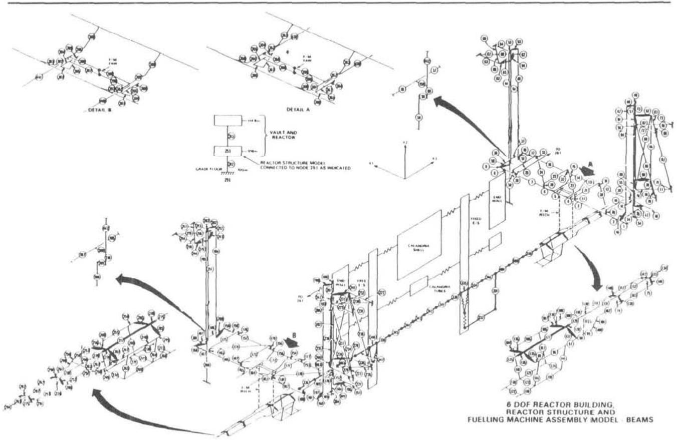
Figure 5b: Fuelling machine dynamic analysis model.
