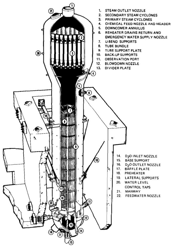
Figure 3a: Steam generator for 600 MW(e) NPs.
