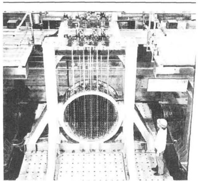
Figure 7a: CANDU core seismic test 1/5 scale model.
