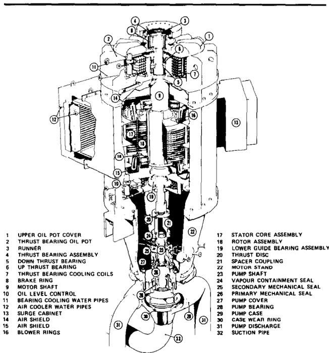
Figure 2a: Heat transport system pump.
