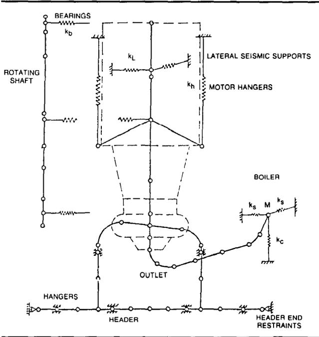
Figure 2b: Schematic dynamic model of pump.
