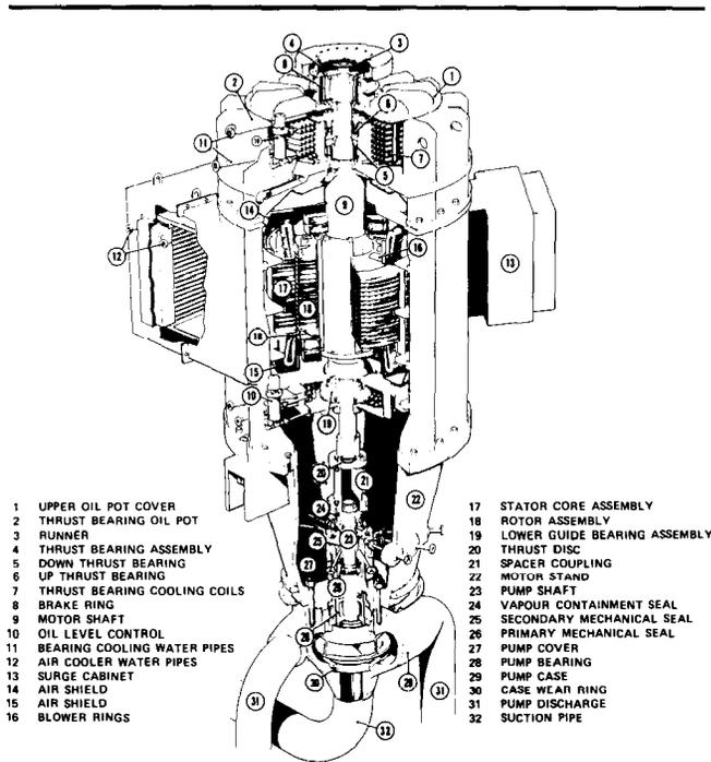
Figure 2a: Heat transport system pump.
