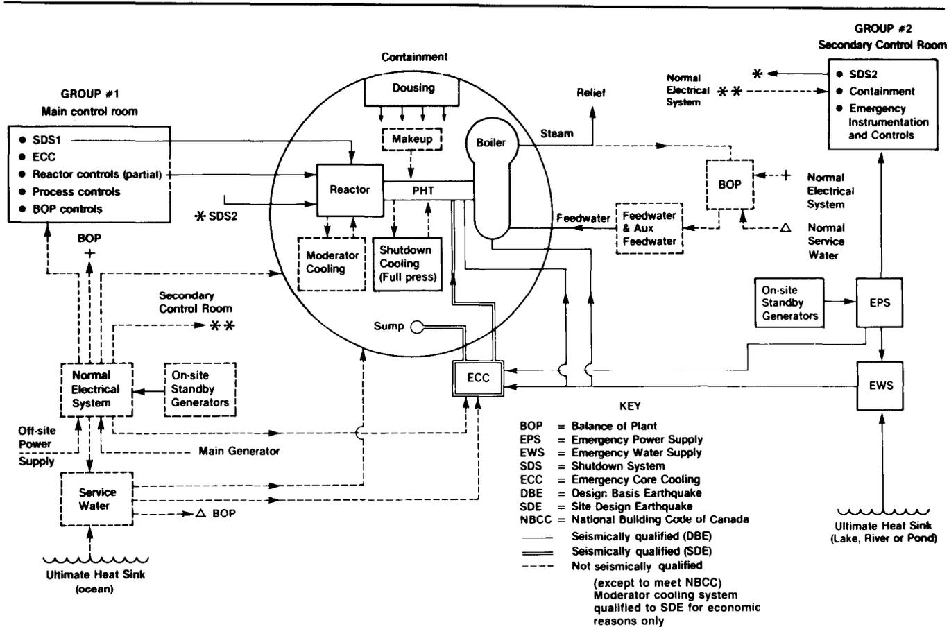
Figure 1: Seismic qualification and system separation for a CANDU 600 NPP on an ocean site.
